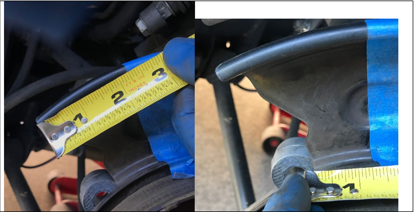
Here is a picture of the dust shield on the passenger side and how far the cut needs to clear.
