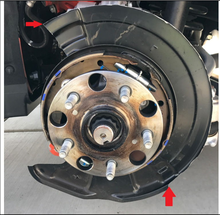
Here is a picture of the dust shield on the passenger side and how far the cut needs to clear.
